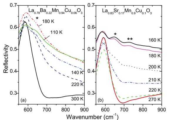
Fig. 2. Temperature dependence of the infrared reflectivity of (a)  $\text{La}_{0.78}\text{Ba}_{0.22}\text{Mn}_{0.94}\text{Cu}_{0.06}\text{O}_3$ , and (b)  $\text{La}_{0.83}\text{Sr}_{0.17}\text{Mn}_{0.9}\text{Cu}_{0.1}\text{O}_3$  samples.
