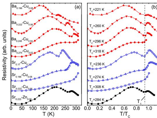
Fig. 1. (a) Temperature dependence of the electrical resistivity of the  $\text{La}_{1-x}[\text{Sr}(\text{Ba})]_x\text{Mn}_{1-z}[\text{Cu}(\text{Zn})]_z\text{O}_3$  samples. (b) The same results represented in the temperature scale normalized to  $T_C$ . Dashed line denotes the value  $T_1/T_C = 0.93$ .
