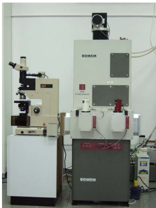
BOMEM DA8 with new InSb and Si detectors as well as Spectra-tech IR-PLAN advanced analytical microscope
