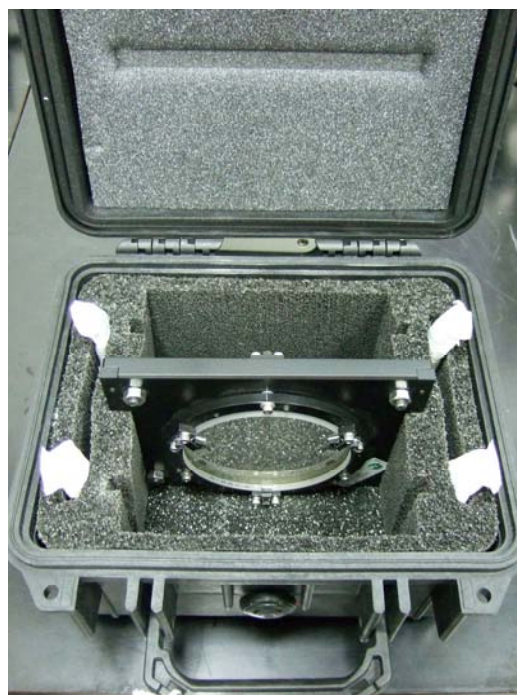
The new Quartz beamsplitter for the range 4000\text{--}25000\text{ cm}^{-1}
