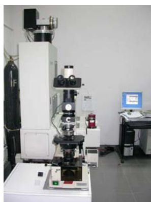
Figure 2. IR Plan microscope mounted on Bomem DA8 spectrometer
